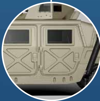
Ballistic protection for floor and side panels
