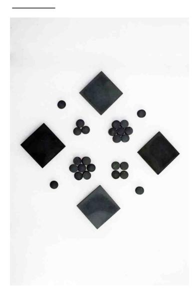
Diamonds are the hardest naturally occurring mineral, with a rating of 10 on the Mohs hardness scale. Although synthetically produced, silicon carbide (SiC) comes very close at a rating of 9 next to diamond.
