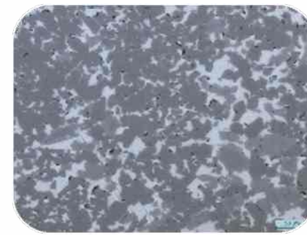
CUMI Rb(SiC+B 4 C) (Reaction Bonded Silicon Carbide + Boron Carbide)
